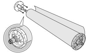
The roll media is locked in place by the roll holder.
